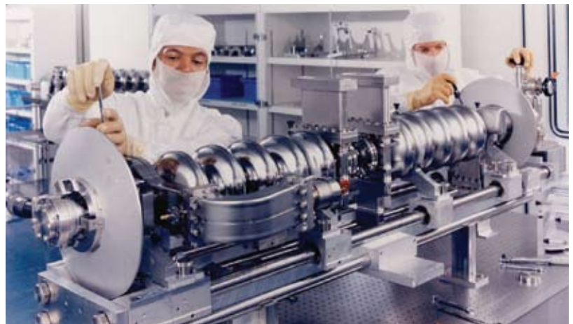
Nobium Cavity Pair Assembly in Clean Room
