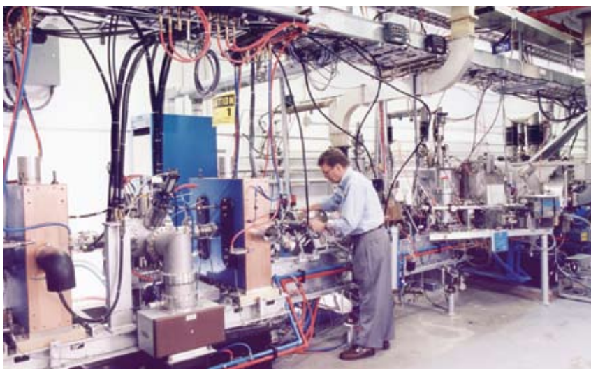
Continuous electron beam is injected into the accelerator tunnel
