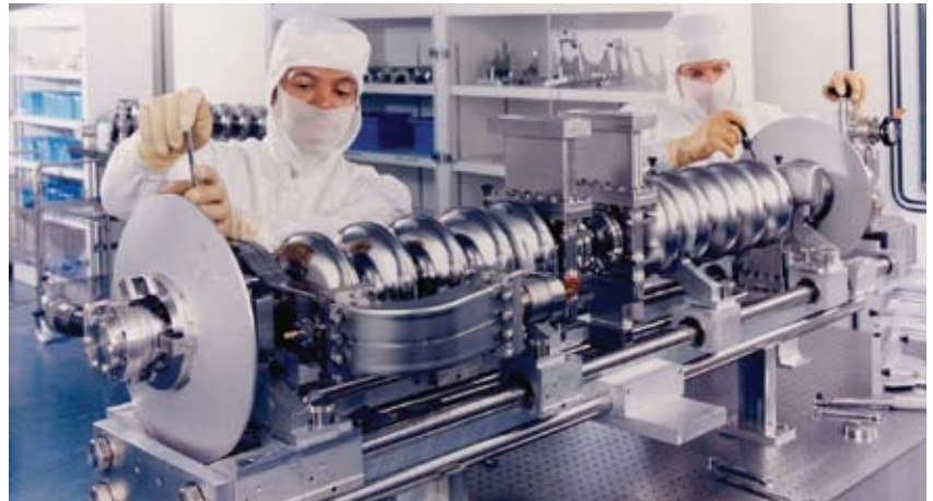
Nobium Cavity Pair Assembly in Clean Room
