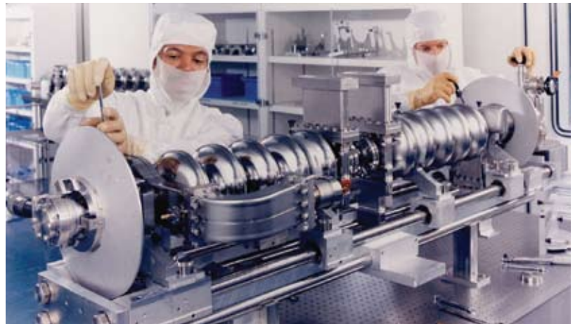
Nobium Cavity Pair Assembly in Clean Room
